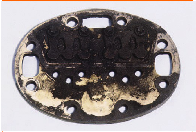
Figure 4 — Valve Plate with Oil Breakdown Deposits
