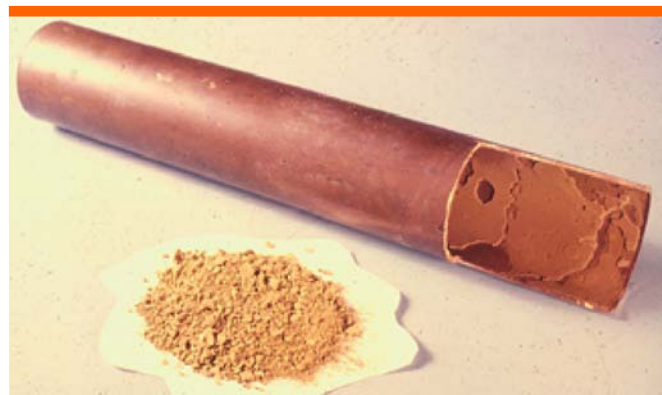
Figure 1 —Oil Breakdown Deposits on Inner Walls of System Piping
