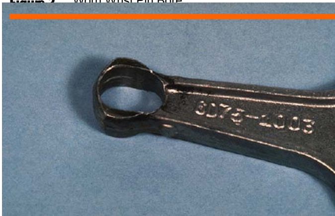
Figure 2 — Worn Wrist Pin Bore
